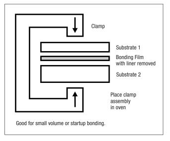
**Hydraulic or Mechanical Press Bonding**
