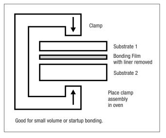
**Hydraulic or Mechanical Press Bonding**
