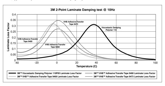
Viscoelastic Damping Polymer 110 VHB<sup>™</sup> Adhesive Transfer Tapes 9460 • 9469 • 9473
