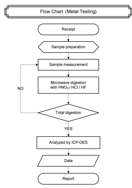
\*\* Remarks : The samples were dissolved totally by pre-conditioning method according to above flow chart.
